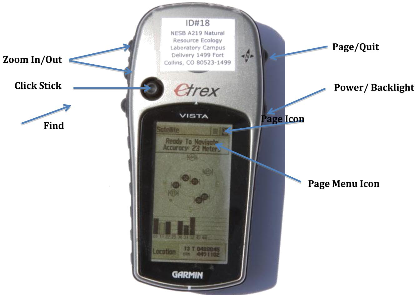
**Power/Backlight:** Lower Right Button. Press and hold till unit turns on
